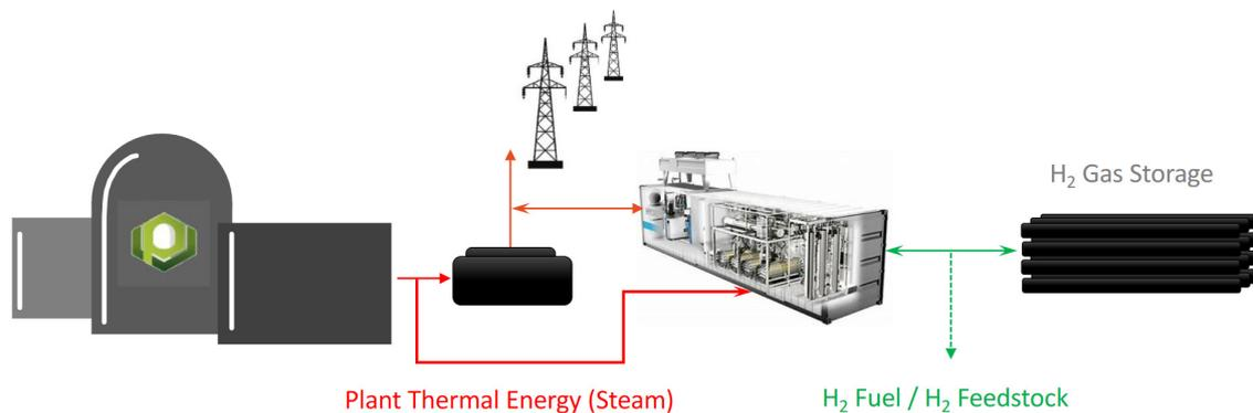
Fig. 7 - Existing nuclear power plant being utilized to support efficient hydrogen production via steam electrolysis at a site within the US<sup>30</sup>
