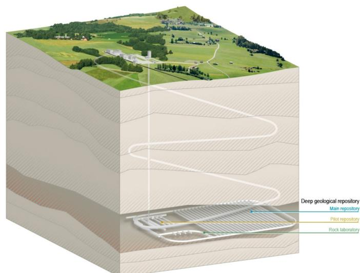
Figure 1: Illustration of a potential DGR design – Swiss Federal Safety Inspectorate (ENSI)
