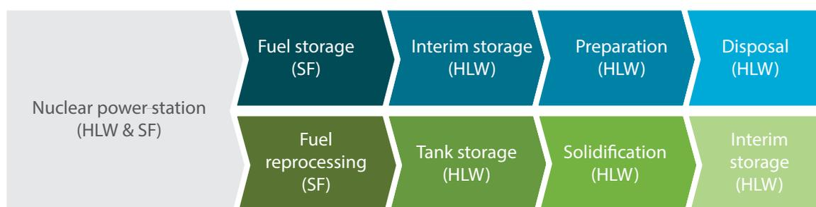
Figure 3: Generation, conditioning, storage, and disposal of SF/HLW<sup>3</sup>
