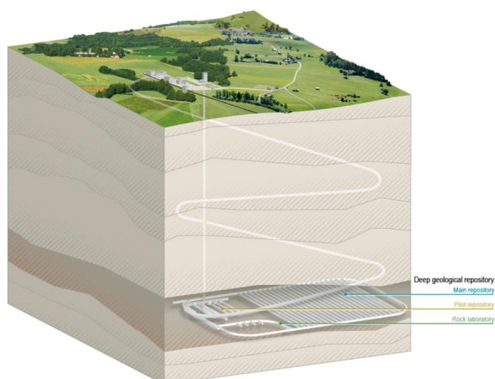
Figure 1: Illustration of a potential DGR design – Swiss Federal Safety Inspectorate (ENSI)
