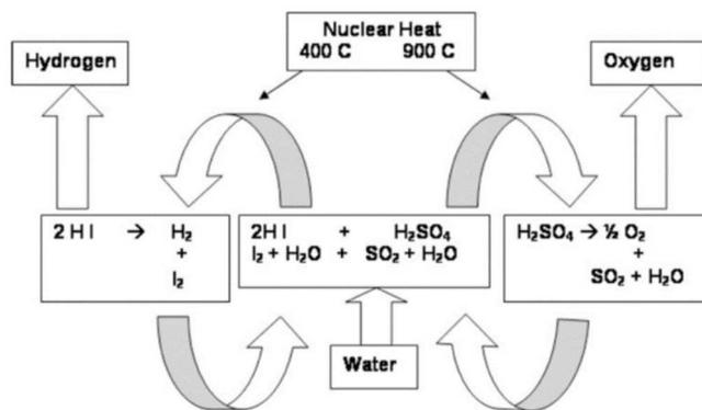
Figure 15 : the sulfur-iodine thermochemical cycle for hydrogen production
