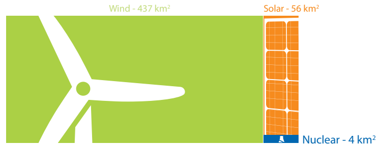
Land required by different energy sources to match the amount of electricity produced by a 1,800 MW nuclear power plant.
